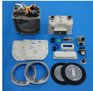
Disassembled gas meter
