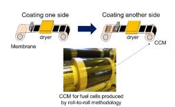
Catalyst coating technology for production of CCM for fuel cells
