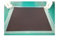
CCM over 800 cm<sup>2</sup> for water electrolysis
