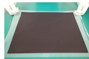
CCM over 800 cm 2 for water electrolysis
