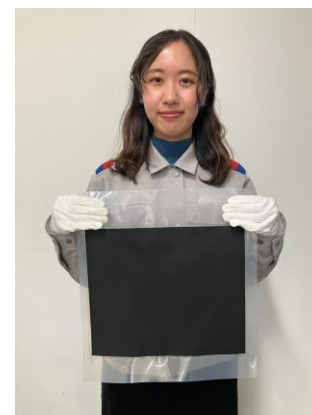
CCM over 800 cm 2 for water electrolysis
