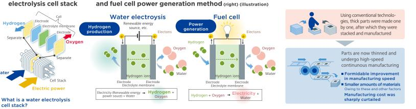
It comprises of multiple stacks of thin parts (cells) that produce hydrogen and oxygen through water electrolysis (fuel cells have a reverse reaction).
