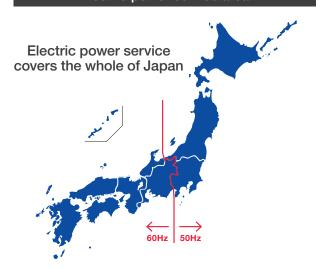
All electric power grids across the whole of Japan, from Hokkaido in the northeast to Kyushu in the southwest, are connected by power distribution lines. This infrastructure enables power exchange (lending) across the conventional barriers between individual power companies, and supports the stable supply of electricity and efficient operation of power generation facilities.
