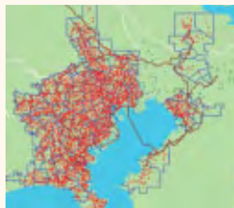
Distribution of Earthquake Sensors (Red dots: Tokyo Gas seismometers Blue frameworks: Disaster prevention blocks)
