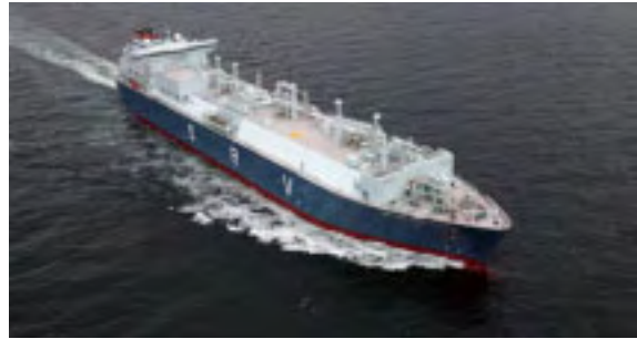
LNG Carrier with Onboard Regasification Equipment
