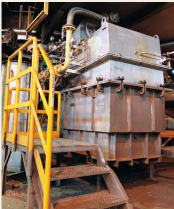
Aluminum Melting Furnace
