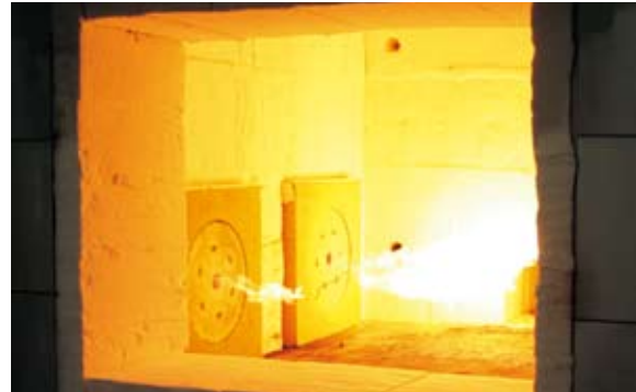
Regenerative Burner System This system efficiently recovers the high-temperature exhaust gas from industrial furnaces and uses it to preheat the air utilized for combustion. This system is drawing attention as an effective means to save energy and reduce CO 2 emissions.
