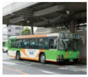
Natural gas vehicles, which produce reduced NOx emissions, include this city bus.
