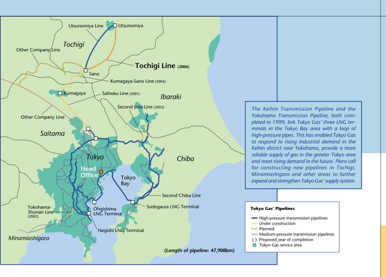
produced natural gas is used as a feedstock in the Utsunomiya service area. When complete, the new Tochigi Pipeline will sharply increase our transportation capacity to this area, enabling the supply of gas derived using LNG from terminals in Tokyo Bay. Our objective is to also capture large-volume demand from industrial areas neighboring the new pipeline. About 70 km in length, the new pipeline is slated for completion in 2006.
