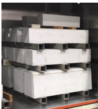
Test manufactured CO 2 -absorbing Concrete Products (Ground boundary blocks)
