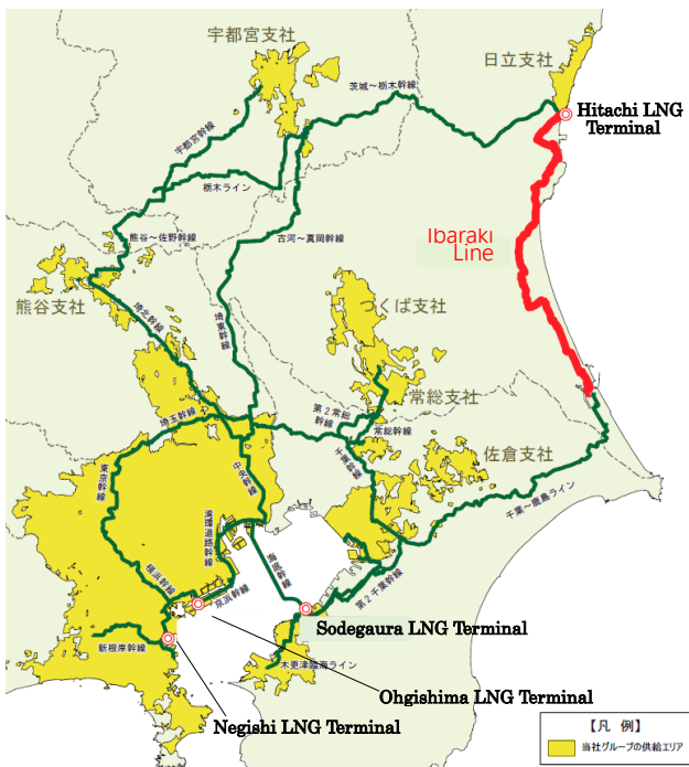
Tokyo Gas’s High-pressure Gas Pipelines
