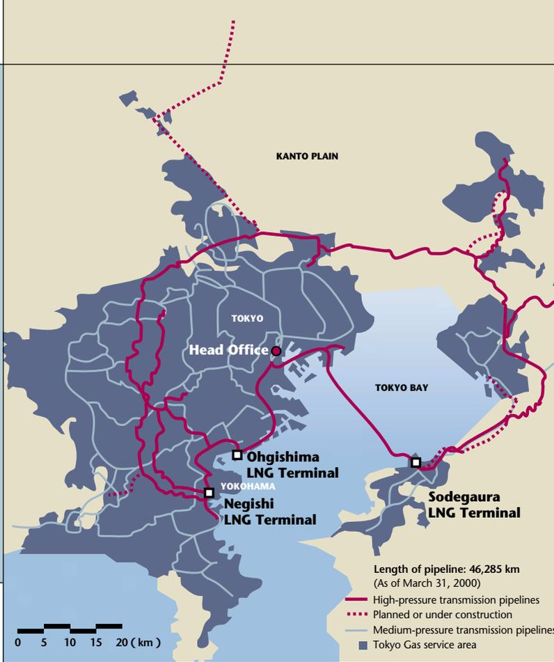
The Negishi, Sodegaura and Ohgishima LNG terminals are now connected by a loop of high-pressure pipes following the December 1999 completion of the Keihin and Yokohama transmission pipelines. This means Tokyo Gas can start responding to rising industrial demand in the Keihin district near Yokohama, provide a more reliable supply of gas in the greater Tokyo area and meet rising demand in the future.
