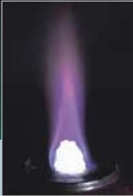
Methane hydrate combustion: Tokyo Gas is pushing ahead with research into technologies for using methane hydrate, which is expected to become a major source of energy in the 21st century.
