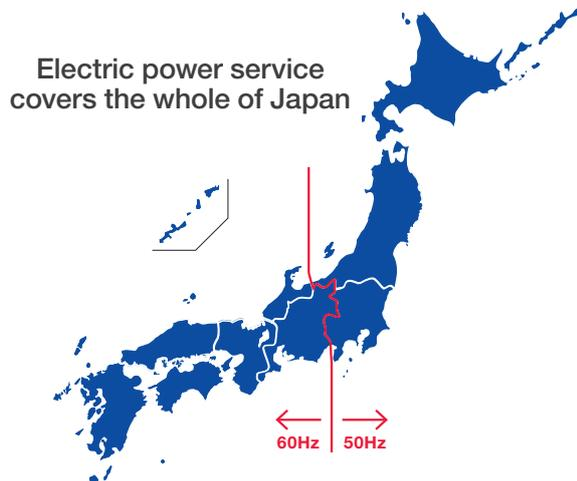
All electric power grids across the whole of Japan, from Hokkaido in the northeast to Kyushu in the southwest, are connected by power distribution lines. This infrastructure enables power exchange (lending) across the conventional barriers between individual power companies, and supports the stable supply of electricity and efficient operation of power generation facilities.
