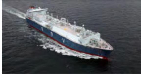
LNG Carrier with Onboard Regasification Equipment
