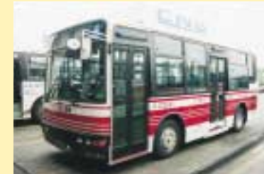
A natural gas vehicle with very low NO x emission levels (community bus in Setagaya Ward, Tokyo)
