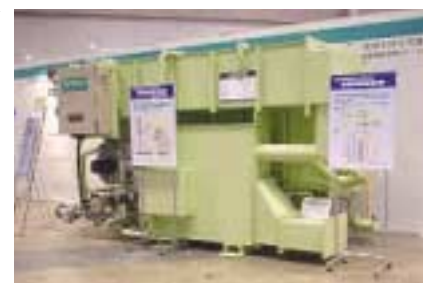
High-efficiency absorption-type chiller-heater
