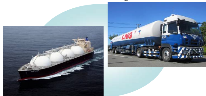
LNG Supply by Means of Lorries and Coastal and Ocean-Going Tankers
